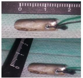
**Fig 1:** the designed carbonated stainless steel shield connected to a silk thread passing through a hole in its middle near upper edge of nearly 1.5 cm length and 0.6 cm width.
