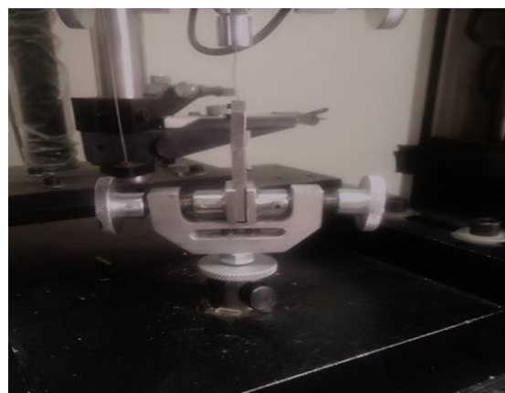
Fig. 1. Universal Tensile Testing Machine STM-20. When the load cell (attached to the upper clamp) registers tension the lower clamp moves downward.
